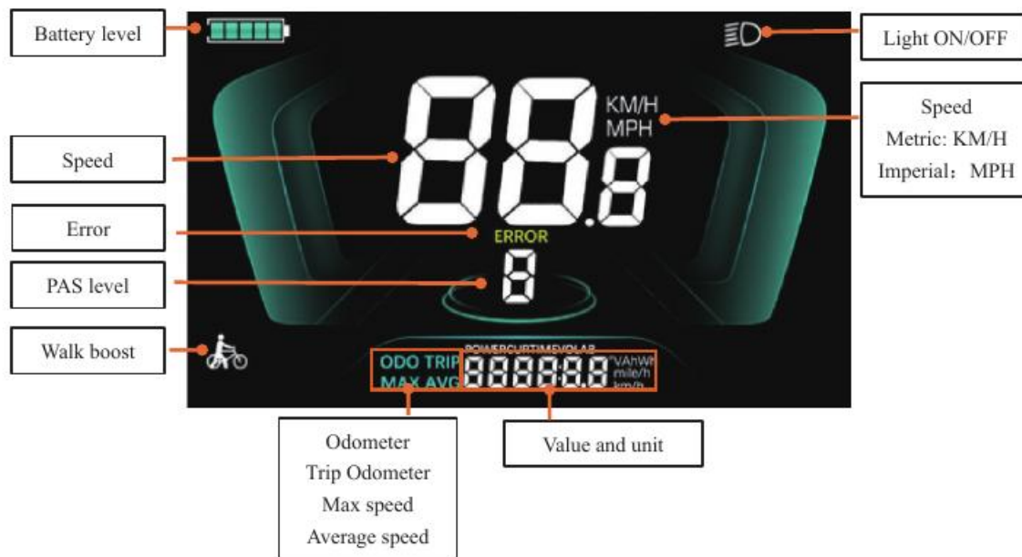
Figure 4-1 YL61F-D functional area distribution interface
