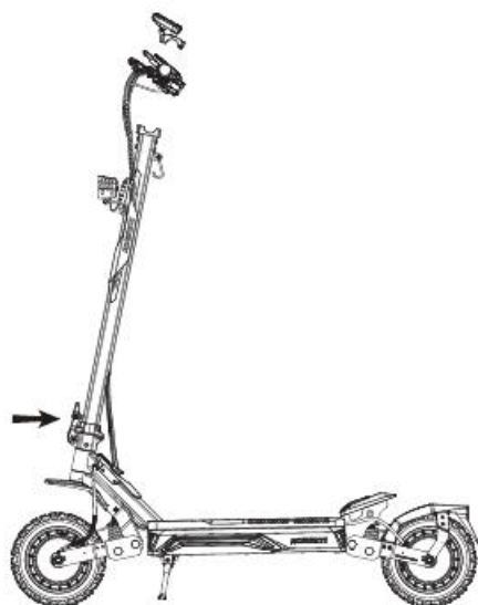
3. Lock the folding mechanism. (Please refer to the unfolding steps.)
