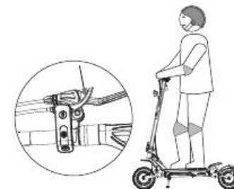
4. When the scooter starts to run steadily, make both of your feet stand on the scooter. Accelerate the scooter by pressing the thumb throttle slightly.
