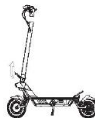
1.Pull out the bracket and fix the folding switch.
