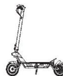
2.Insert the T-shaped front-end into the upright pole.
