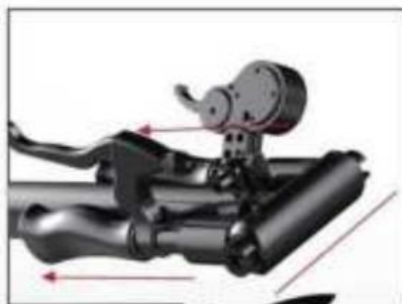
Step 3: bend the handle downward
