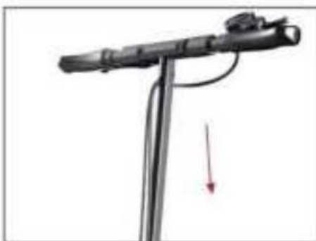
Step 5: adjust T-shaped tube downward Krok 5: posuňte T-stĺpik nadol
