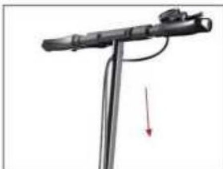
Step 5: adjust T-shaped tube downward
