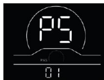
Fig. 4-5 Speed Sensor Setting Interface
