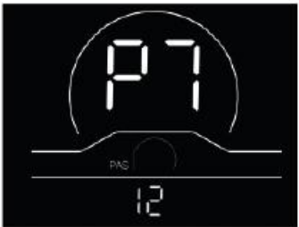
Fig. 4-7 Assistance Sensor Setting Interface
