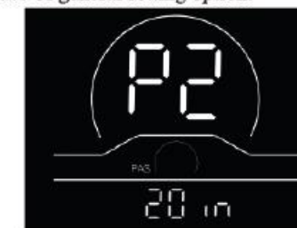
Fig. 4-2 Wheel Diameter Setting Interface
