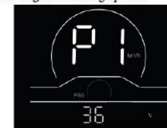
Fig. 4-1 Rated Voltage Setting Interface
