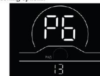
Fig. 4-6 Current Limit Setting Interface
