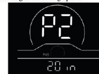
Fig. 4-2 Wheel Diameter Setting Interface
