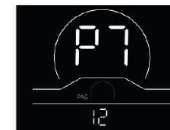
Fig. 4-7 Assistance Sensor Setting Interface
