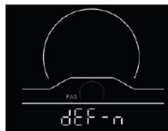
Fig. 3-1 Factory Reset Interface
