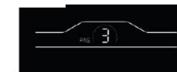
Fig. 2-3 Assist Level Switching Interface
