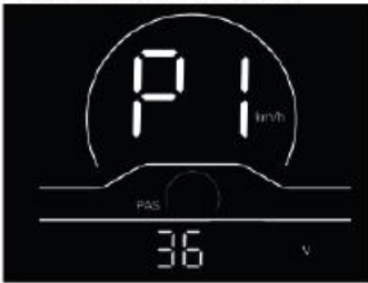
Fig. 4-1 Rated Voltage Setting Interface
