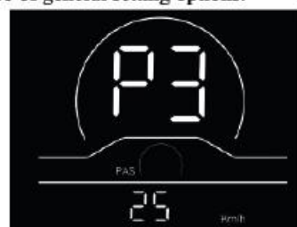
Fig. 4-3 Speed Limit Setting Interface
