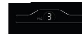
Fig. 2-3 Assist Level Switching Interface
