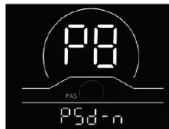
Fig. 4-8 Power-on Password Setting Interface
