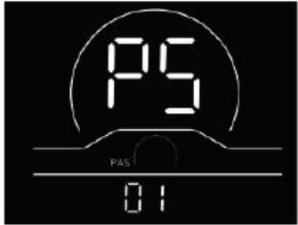
Fig. 4-5 Speed Sensor Setting Interface
