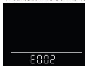
Fig. 2-5 Error Code Indicator Interface
